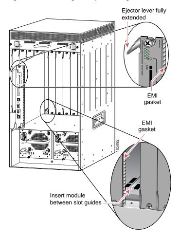
Gap between the module EMI gasket and the module above it
